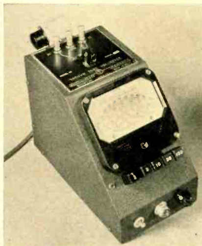
Fig. 8. Typical v-t voltmeter (Courtesy Measurements Corp.)
